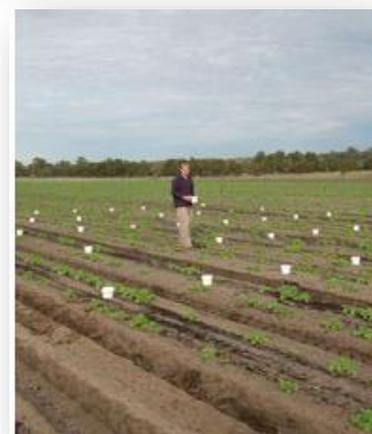
A system with poor distribution uniformity will require additional irrigation to be applied to ensure the minimum water application is achieved at the driest location. For example, a system running with a pressure drop 50 kPa will decrease the distribution uniformity and the irrigation will need to be run for an additional 10% resulting in an equivalent increase in water consumption.
