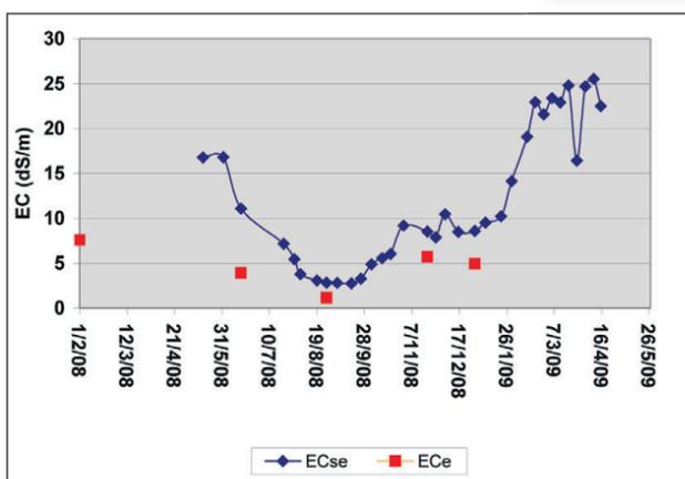
Figure 3: Weighted saturated paste (ECe) and soil solution extract (ECse) measurement. Standard FAO weighting percentages were used. (Source ICMS 2009)
