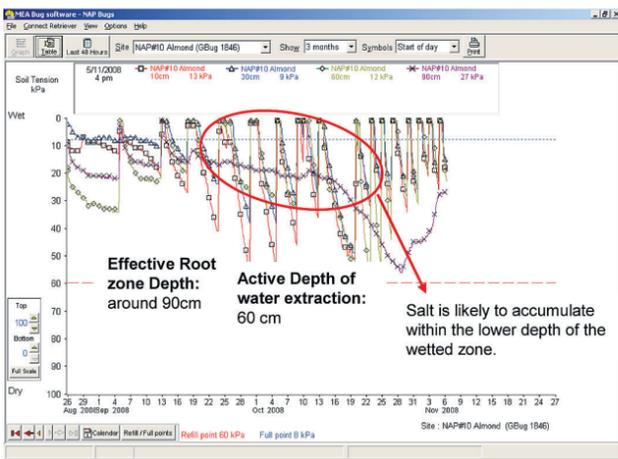
Figure 2: Interpreting salt movement using soil water monitoring data. (Source ICMS 2009)
