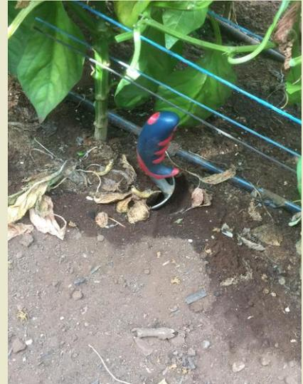
Sampling with a trowel near the plant stems to collect both soil and roots.
